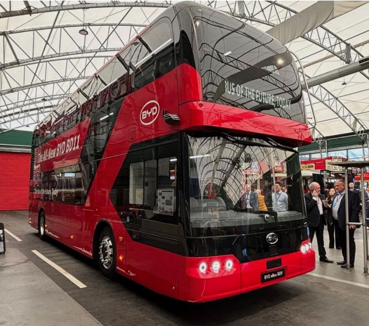
BYD bus, battery 520 kWh, range 400 km
